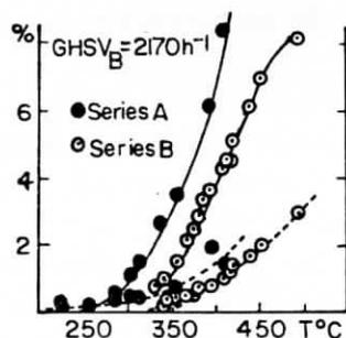
Fig. 2. Yields of combustion products (—) and total C<sub>4</sub> olefins (----) as a function of temperature. C<sub>4</sub>H<sub>10</sub>:O<sub>2</sub>:N<sub>2</sub>=20:15:65 mol %
