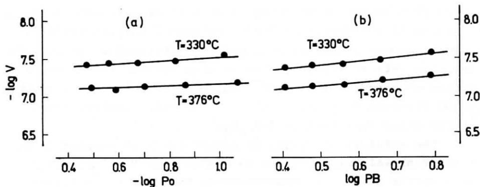
Fig. 2. Dependence of the reaction rate on oxygen (a) and n-butane (b) partial pressure
