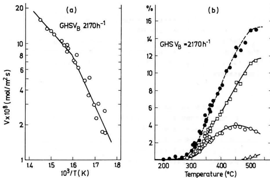
Fig. 1. (a) Arrhenius plot. (b) Conversion of n-butane(---) and yields (—) in total  $\text{C}_4$  olefins (●), combustion (□) and cracked products (Δ)
