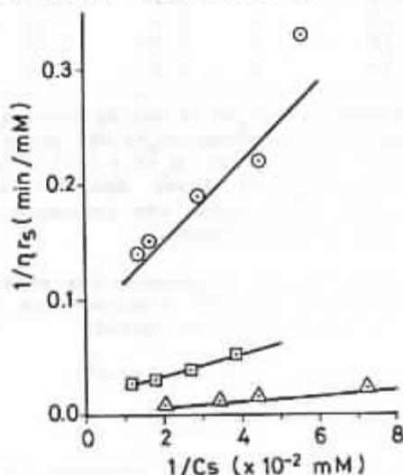
Fig.2 : Comparison of experimental results (open symbols) with values calculated according to Eqn. (18) (trace lines) for sucrose inversion by immobilized yeast cells (Toda and Shoda, 1975). Maximum rate  $V_m$  ( $\mu\text{mol}/\text{min.cm}^3$ ):  $\circ$  12;  $\square$  57;  $\triangle$  455.  $R_p=0.047$  cm;  $K_m=38$  mM;  $D_e=4 \cdot 10^{-4}$   $\text{cm}^2/\text{min}$ . Abbreviations are as in Tables 1 and 2.
