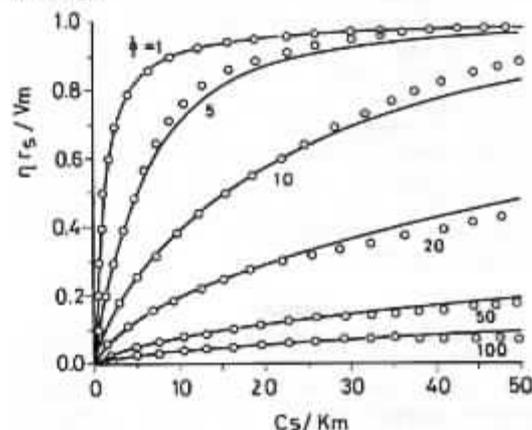
Fig.1 : Plots of the normalized rate of reaction  $\eta r_s/V_m$  against the dimensionless substrate concentration  $C_s/K_m$  at different values of  $\phi = R_p(V_m/D_e.K_m)^{1/2}$ . Trace line draw from Eqn. (18).  $\circ \circ \circ$  Numerical calculation (Horvarth and Engasser, 1974). Abbreviations are as in Tables 1 and 2.
