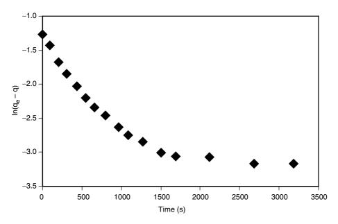
Figure 1. Test of the pseudo-first-order model for describing the kinetics of phenol adsorption from aqueous solution onto peanut shell activated carbon. Experimental conditions:  $C_0 = 0.511 \text{ mmol/l}$ ; D = 1.67 g/l;  $d_p = 0.21 \text{ mm}$ .
