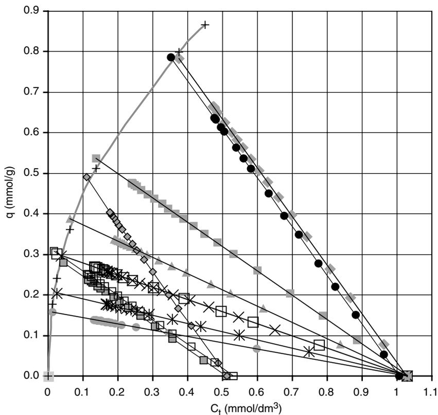
**Figure 9.** Operating lines and equilibrium adsorption isotherm at various initial phenol concentrations, carbon dosages and particle sizes. Data points relate to the following solid/liquid ratios:  $\blacklozenge$ , 0.83;  $\blacksquare$ , 1.67;  $\blacktriangle$ , 2.50;  $\times$ , 3.33;  $*$ , 5.0;  $\bullet$ , 6.53;  $+$ , equilibrium values. Open symbols relate to a particle size diameter,  $d_p$ , of 0.45 mm; filled symbols relate to a particle size diameter of 0.21 mm.
