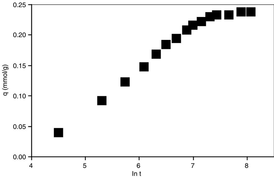
**Figure 4.** Test of the Elovich equation for describing the kinetics of phenol adsorption from aqueous solution onto peanut shell activated carbon. Experimental conditions:  $C_0 = 0.511$  mmol/l;  $D = 1.67$  g/l;  $d_p = 0.21$  mm.
