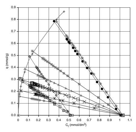
Figure 9. Operating lines and equilibrium adsorption isotherm at various initial phenol concentrations, carbon dosages and particle sizes. Data points relate to the following solid/liquid ratios:  $\blacklozenge$ , 0.83;  $\blacksquare$ , 1.67;  $\blacktriangle$ , 2.50;  $\times$ , 3.33; \*, 5.0;  $\spadesuit$ , 6.53; +, equilibrium values. Open symbols relate to a particle size diameter,  $d_p$ , of 0.45 mm; filled symbols relate to a particle size diameter of 0.21 mm.
