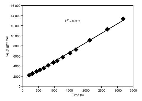
Figure 2. Test of the pseudo-second-order model for describing the kinetics of phenol adsorption from aqueous solution onto peanut shell activated carbon. Experimental conditions:  $C_0 = 0.511 \text{ mmol/l}$ ; D = 1.67 g/l;  $d_p = 0.21 \text{ mm}$ .
