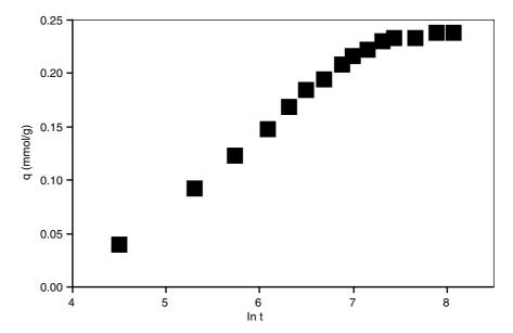
Figure 4. Test of the Elovich equation for describing the kinetics of phenol adsorption from aqueous solution onto peanut shell activated carbon. Experimental conditions:  $C_0 = 0.511 \text{ mmol/l}$ ; D = 1.67 g/l;  $d_p = 0.21 \text{ mm}$ .
