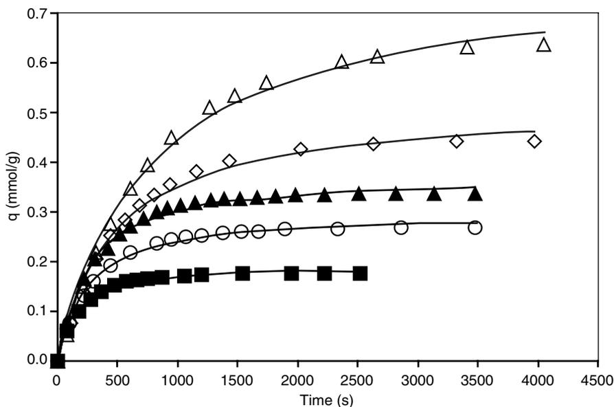
**Figure 5.** Variation with time of the capacity of peanut shell activated carbon towards the adsorption of phenol from aqueous solution at the following solid/liquid ratios:  $\Delta$ , 0.83;  $\diamond$ , 1.67;  $\blacktriangle$ , 2.50;  $\circ$ , 3.33;  $\blacksquare$ , 5.00. Open symbols relate to a particle size diameter,  $d_p$ , of 0.45 mm; filled symbols correspond to a particle size diameter of 0.21 mm. Experimental conditions:  $C_0 = 1.03$  mmol/l; agitation speed = 500 rpm.
