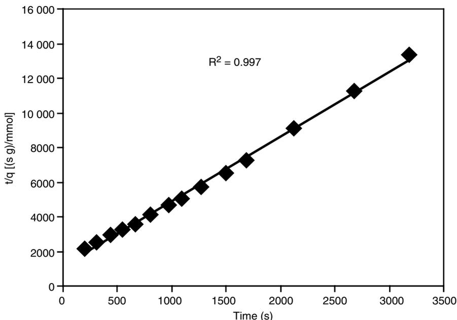
**Figure 2.** Test of the pseudo-second-order model for describing the kinetics of phenol adsorption from aqueous solution onto peanut shell activated carbon. Experimental conditions:  $C_0 = 0.511$  mmol/l;  $D = 1.67$  g/l;  $d_p = 0.21$  mm.
