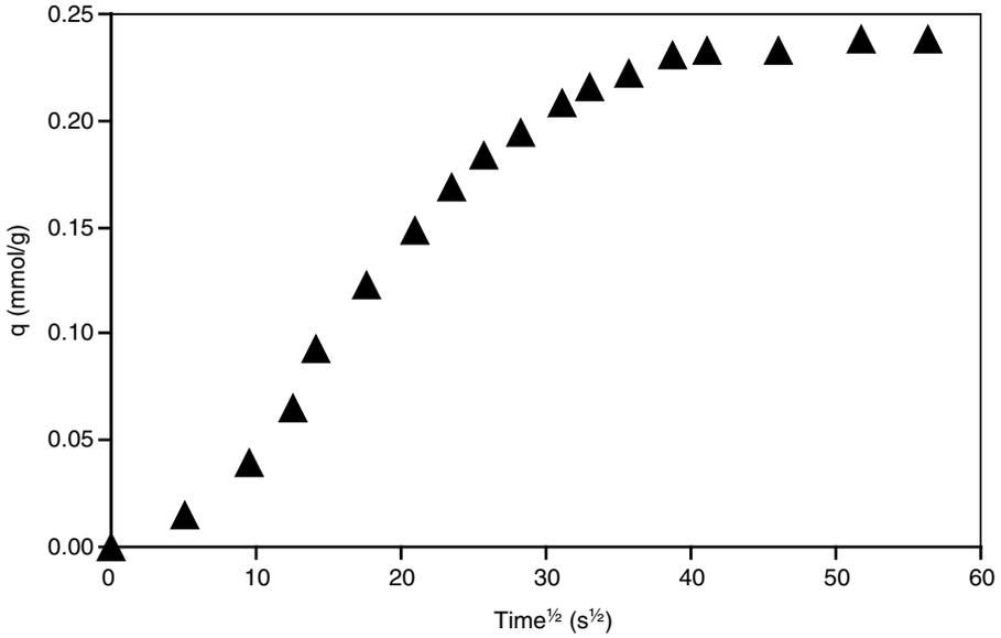
**Figure 3.** Test of the intraparticle diffusion model for describing the kinetics of phenol adsorption from aqueous solution onto peanut shell activated carbon. Experimental conditions:  $C_0 = 0.511$  mmol/l;  $D = 1.67$  g/l;  $d_p = 0.21$  mm.
