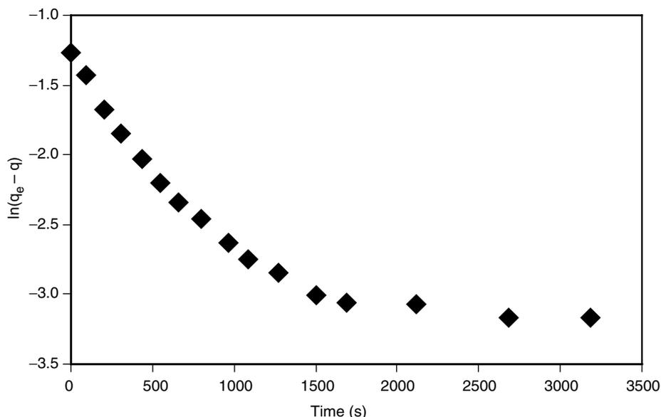
**Figure 1.** Test of the pseudo-first-order model for describing the kinetics of phenol adsorption from aqueous solution onto peanut shell activated carbon. Experimental conditions:  $C_0 = 0.511$  mmol/l;  $D = 1.67$  g/l;  $d_p = 0.21$  mm.
