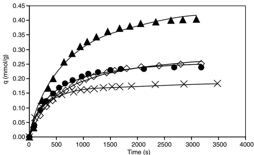
**Figure 6.** Variation with time of the capacity of peanut shell activated carbon towards the adsorption of phenol from aqueous solution at the following solid/liquid ratios: ▲, 0.83; ◇, 1.67; ●, 1.67; ×, 2.50. Open symbols relate to a particle size diameter,  $d_p$ , of 0.45 mm; filled symbols relate to a particle size diameter of 0.21 mm; × symbols relate to a particle size diameter of 0.14 mm. Experimental conditions:  $C_0 = 1.03$  mmol/l; agitation speed = 500 rpm.
