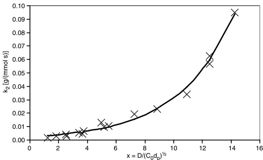
**Figure 8.** Correlation between the rate constant  $k_2$  [g/(mmol s)] and the quantity  $x = D/(C_0 d_p)^{1/2}$ , where  $d_p$  is the particle diameter expressed in mm, for the adsorption of phenol from aqueous solution onto peanut shell activated carbon.
